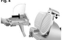
At the same time, loosen the carriage adjustment knob. If you cannot fully loosen it, pull the carriage once more towards the carriage adjustment knob until there is an audible click of protection device.
