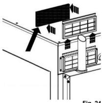
To maintain correct temperature of the electronic elements of the device the fan should be cleaned periodically, **at least once a month**.
