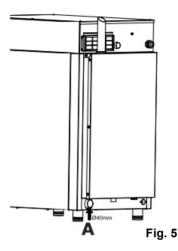
Water flowing from the device drain may be hot (90°C), therefore the drain hoses should be resistant to such temperature.
