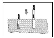
Stick the metal dowels with the attachment screws into the drilled holes in the ground as illustrated.
