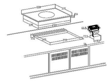
4. Provide sufficient ventilation around the appliance and make sure that the ventilation holes are not obstructed.
