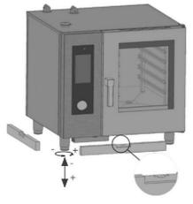
Position the appliance vertically — to this end, the height of adjustable feet is set with a spirit level, as indicated in Fig. 2.
